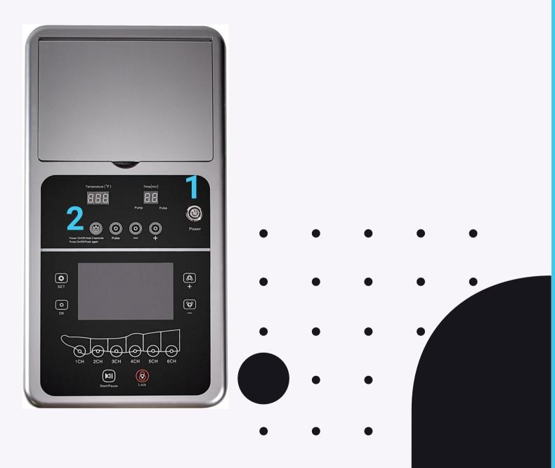
Press Power button on right corner (metal button) in order to switch on the device
